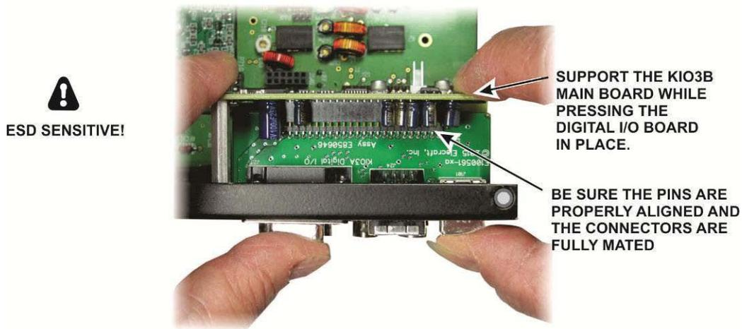
Figure 7. Installing the KIO3 Digital I/O Board.
