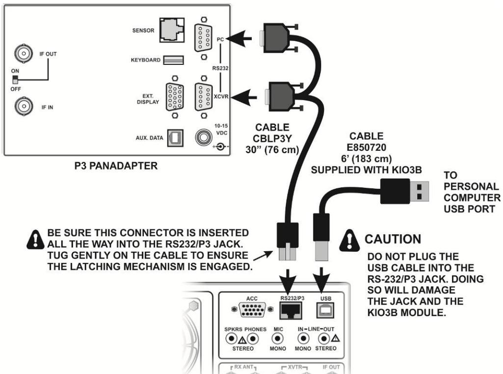
Figure 14. P3 Panadapter Cabling for USB Computer Interface.
